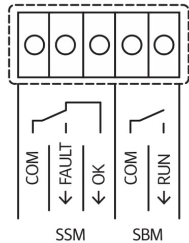
SSM: Collective fault signal (NC contact in accordance with VDI 3814, load capacity 1 A, 250 V ~)
